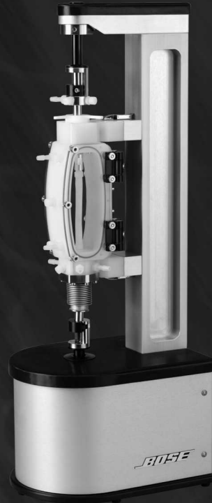
Pulsatile BioDynamic™ Test Instrument for Vascular Grafts
