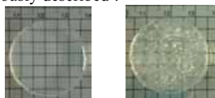
Figure 1. Morphology of hydrogel (G1) and porous hydrogel (G1A) were stored after 24 h in the water
