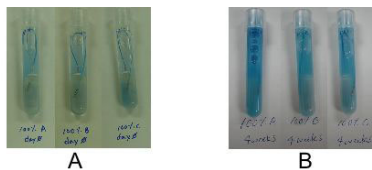
Figure 1: Figure 1A: Pump assemblies inside collection vessels on day 0. After four weeks, particles can be visualized by the blue coloration of the collection suspensions (Figure 1B).
