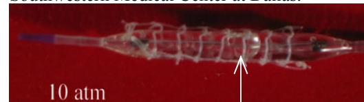
Fig 1. During expansion inner coils are extended axially and permanently twisted (arrow) since stresses in torsion exceed the elastic limit.
