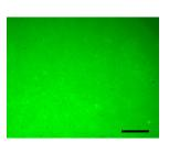
Fig. 1: Uniform deposition of microgel-based coatings on PET. Microgel particles were covalently immobilized onto PET and labeled with FITC via pendant amine groups. Scale bar 20 um.
