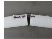
Figure 3: Example of plate failure – Exp #2
