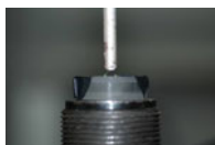
Figure 3. Fixture of thermocoil for radial strength test
