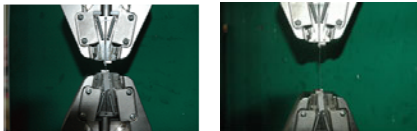
Figure 2. Photographs of tensile test with holding jaws
