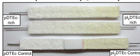
Fig. 2. Rod-shaped pDTEc/pI 2 DTEc scaffold libraries are at top of image. Control pDTEc (left) and pI 2 DTEc (right) scaffolds are at bottom. Stainless steel wires were incorporated into the scaffolds for reinforcement and to ease handling. Gradients range from 5 % to 83 % pDTEc by mass.
