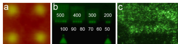
Figure 1. Amine-terminated PEG nanopatterns for actin polymerization. (a) AFM image of \sim 100 nm diameter crosslinked NH 2 -terminated 8-arm PEG patterns. (b) Amine reactive dye bound to polymer nanopatterns. Diameter sizes are displayed in nm. (c) Image after actin was assembled on the nanopatterns.
