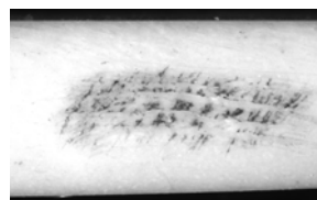
Figure 4. Optical micrograph showing scratches on the surface of a bone specimen stained by Au NPs (dark). The width of the specimen is 5 mm.
