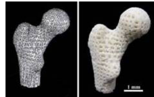
Fig.3 A model of proximal femoral condyle (left) and sintered scaffold (right)
