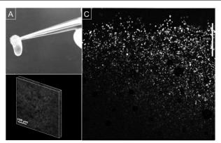
Figure 1: a) microgel scaffold, b) microgel scaffold, 20x, labeled with Dylight-633 c) calcien labeled cells in a microsphere-RGD scaffold
