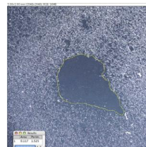
Cells on PyC after Jet Impingement. Sample area in each image: 1sq.mm. L: Autoclaved PyC, R: RFGDT PyC
