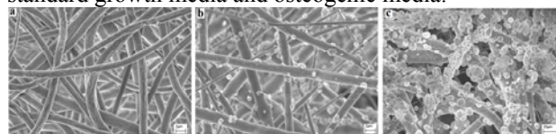
Figure 1: SEM micrographs of electrospun PCL (a) Composite-MC+DMF (b) and Composite-MC (c) immersed in SBF for 28 days
