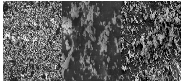
Figure 1: SEM images (X1000) of Spineplex, Cortoss & Heracap, respectively, after 7 days SBF immersion.
