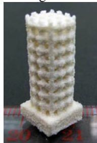
Fig.1 A photo of a sintered scaffold
