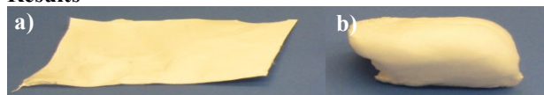
Fig. 1. a) Traditional flat sheet-like nanofibrous ePCL scaffold. b) Cotton ball-like nanofibrous ePCL scaffold.
