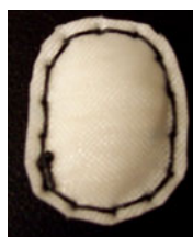
Figure 1: Image of the final assembled nucleus containment prototype. Width between seams is 13 mm and length between seams is 17 mm.
