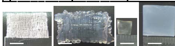
Figure 1. Representative pictures of dressings made by RP (left two) and film casting (right two). Scale bar=5mm.
