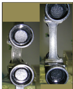
Fig 1: Dogbone shaped gelatin hydrogel before (left) and after (right) tensile test on Instron Material Testing System
