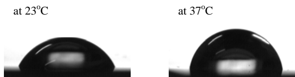
Figure 1. Contact angle images for Si-PNIPAAm surface under different temperatures.
