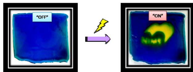
Figure 2. Photographs of P(NIPAAm-CIPAAm) gel containing o -NBA before and after UV irradiation for one minute. UV was irradiated through a mask and the color change of pH indicator in the only exposed region was observed (pH indicator, bromothymol blue; yellow below pH 6.0).
