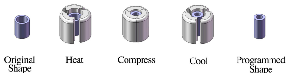
Figure 1: Process for programming shape-memory effect.
