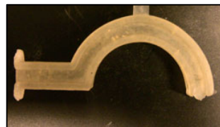
Figure 2: Oropharyngeal airway device molded from novel urethane SMP
