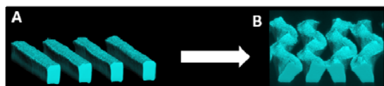
Figure 1: pNIPAAm structures in the collapsed state (A) and the swollen state (B) as imaged by confocal microscopy.
