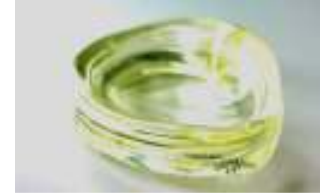
Figure #1: the composite polycarbonate-urethane and UHMWPE meniscal implant developed in the study
