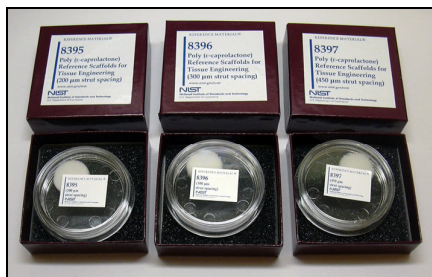
Fig. 1. First generation NIST reference scaffolds currently available and characterized for structure (strut diameter, strut spacing, porosity).
