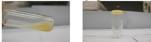
Fig.1. 30wt% hydrogel-HA composite containing 10wt% HA was sol at 4°C (left) and gel at 37°C (right).
