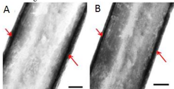
Figure 1. (A) TEM image showing self-assembly of PA on ePCL in the hybrid nanomatrix (ePCL+PA-YK-NO) at 67000x. (B) TEM image of ePCL+PA-YK-NO tilted to 21°, to confirm uniform self assembly. 67000x. Scale bar = 50 nm
