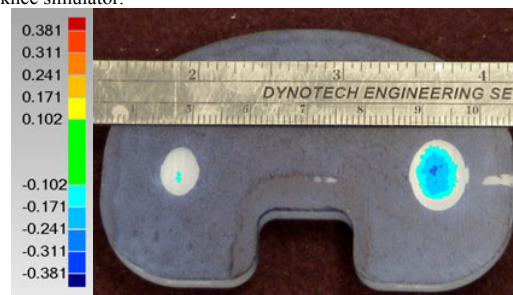
Figure 2. Photograph of contact scars after 1.8 kN load interval showing blue tooling ink removed during articulation. The laser scanner image from the same interval is superimposed, units in mm.
