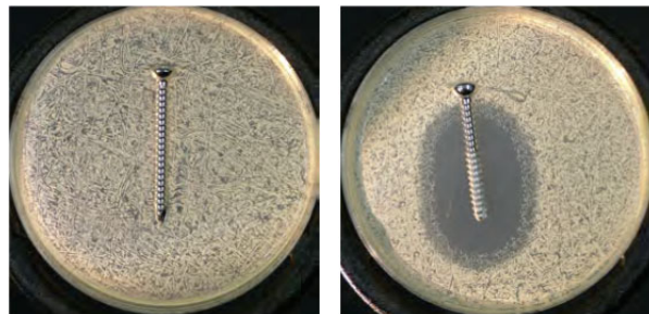
Figure 1: Zone of inhibition results: uncoated (left) and PLLA coated (right)
