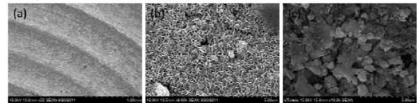
Figure 2. SEM images of (a) coating on PEEK implant; (b) coating crystal structure; (c) a new apatite layer deposited on coating surface after 7 days incubation in cell culture medium
