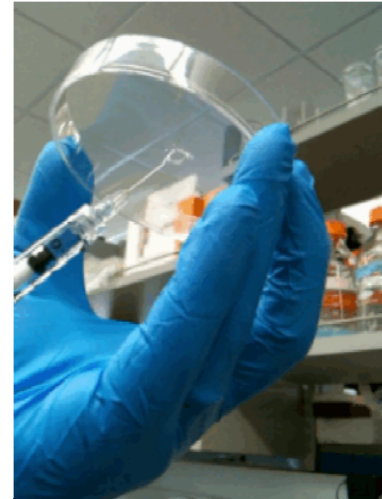
Figure 1. Application of the PEG-DA/HA gel to an inverted surface.
