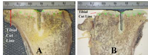
Figure 2. Sample images of image analysis measurement tool. (A) Simplex-HV, (B) Palacos-R
