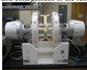
Fig.2 Bose Enduratec Pulsatile Fatigue Tester™ with phantom attached
