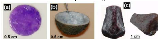
Fig 3. Product range attained by ECOM: (a) compacted collagen II incorporated CS, (b) semispherical scaffolds with HA-collagen (white) and pure collagen (black) layers standing alone, (c) nasal shell layer made by liquid metal nose-like electrodes.
