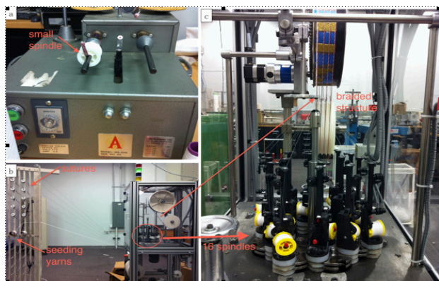
Fig. 1. (a) Winding of yarns for braiding (b) Side view and (c) Front view of 16-spindle braiding machine
