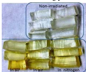
Figure 1. Yellowing of PCU (bottom) vs. non-irradiated PCU (top).
