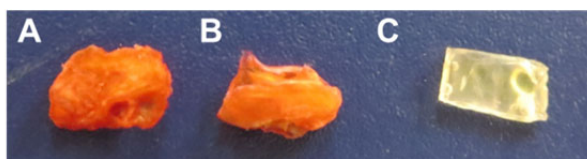
Fig.3. Von Geison staining (red color) for gelatin: (A) 18-PEG400-7G, (B) 18-PEG400-5G, (C) 18-PEG400-0G.
