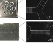
**Figure 1:** (A) Device used for cell migration study. Six satellite reservoirs connect to a central reservoir by different width microchannels (Flower device). (B) Device used for drug study. The cell seeding reservoir (top) is connected to the bottom reservoir via microchannels
